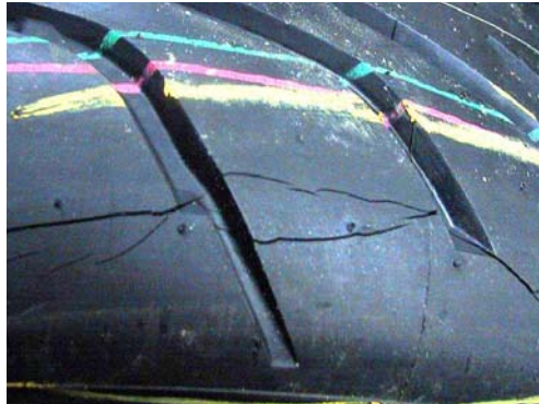
Tread cracking due to low temperatures
